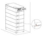
Step 10: Turn the adjusting screws to fix the battery onto the wall by using a wrench.
