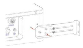
4 Mark the position of 4 holes to be drilled on the wall.
