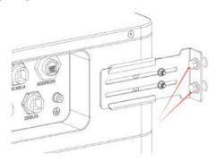
10 Turn the adjusting screws to fix the battery onto the wall by using a wrench.
