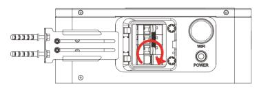
Step2. Hold on "POWER" button for 3 seconds until the indicator becomes green and flashing, which means that the battery enters self-checking.
