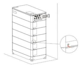
① Insert the expansion screws into the tubes, then fix the mounts onto the wall with expansion screws by using a cross screwdriver.
