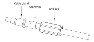
4. Insert the positive and negative cables into the corresponding connectors, and then press the terminal with crimping pliers. After assembling, try to pull back the battery cable to ensure that the terminal is tightly attached in the connector.
