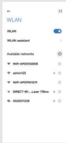
**2** Searching for the corresponding WLAN in the WLAN connection list "WIFI-AP\*\*\*\*\*" (\*represents the last 8 numbers of the inverter SN), and tap connect.
