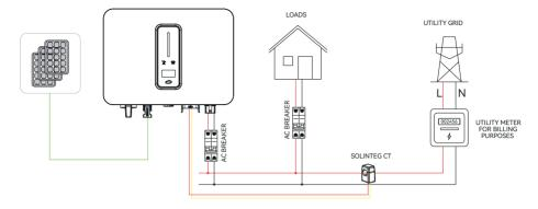
Electrical wiring diagram of export limit
