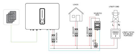
Electrical wiring diagram of export limit & 24 hours load consumption
