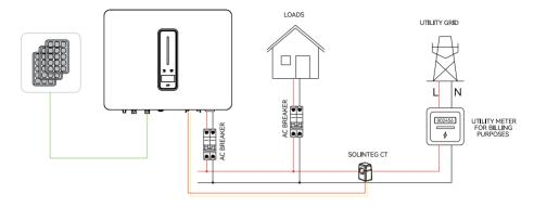
Electrical wiring diagram of export limit
