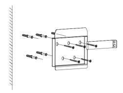
Figure 4-6 Fixing the wall bracket
