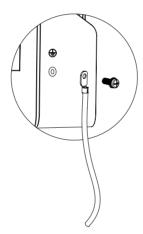
Figure 4-8 Grounding terminal connection
