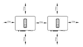
Figure 4-2 Recommended installation spacing
