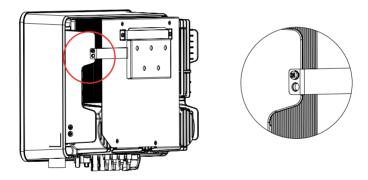
Figure 4-7 Mounting the inverter
