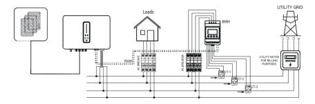
Figure 5-2 Electrical wiring diagram of export limit
