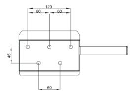
Figure 4-4 Dimensions of wall bracket
