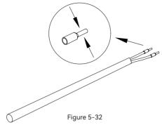
6 Fix all the wires to the terminal plug according to the assignment and tighten to a torque of 1.2+/-0.1N·m with a screwdriver.
