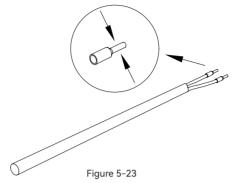
④ Insert the stripped end of the three wires into the appropriate hole of the terminal head.
